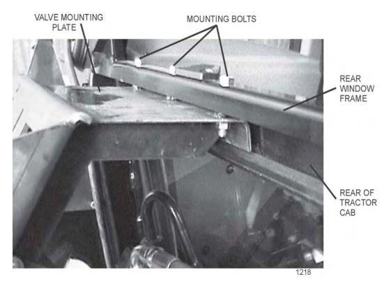
Install the valve mounting plate onto the window frame with the hardware provided. Refer to the parts section for all parts and hardware needed. Align and mount the mounting plate under the window fame with the three capscrews, flatwasher, lockwasher and hex nut. **DO NOT tighten.** Next install the capscrew and lockwasher through the valve mounting strap lower hole into the tractor housing. Once installed tighten all the bolts in the mounting plate.
